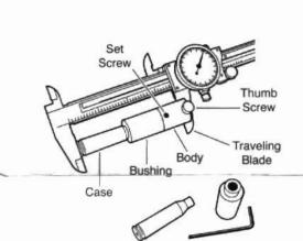
Now, open the caliper and center the case shoulder into the Bushing. Bring the caliper blade to rest on the case head and rotate the case as you remove slack, then take a reading. Be consistent! Most handloaders prefer to carefully "zero" the caliper's indicator on the longest (fire-formed) case. This allows them to gauge the headspace variations from this fire-formed (maximum) case dimension.
