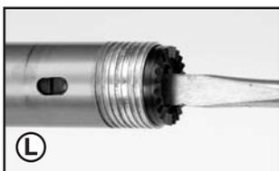
Remove retainer with a screwdriver
