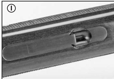
*Forearm release lever on underside of stock*
