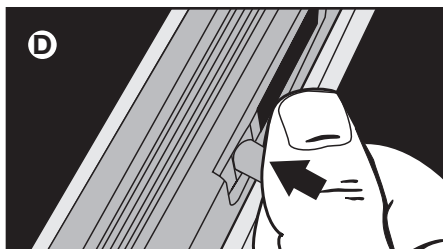
Locking the action open manually
